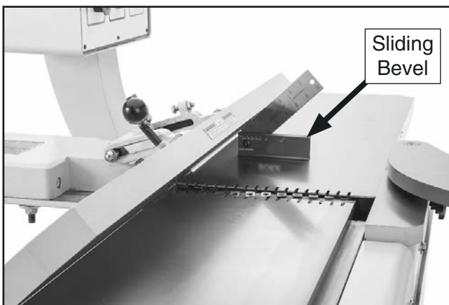
Figure 62. Adjusting fence to 45° inward.
